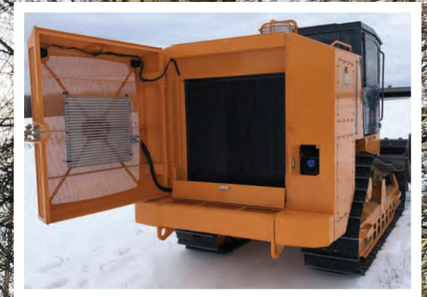
HIGH EFFICIENCY COOLING PACKAGE WITH COARSE FINNS FOR EASY CLEANING
