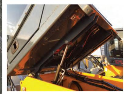
PUSH BUTTON CAB TILT FOR EASY ACCESS TO COMPONENTS & HYDRAULIC OIL FILLING PUMP
